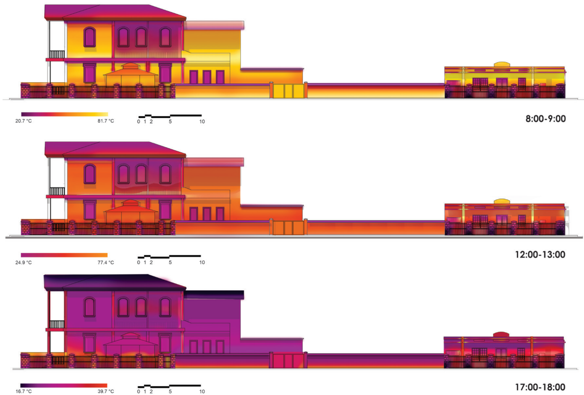
Figure 6: Temperature map of facades. (2024)
