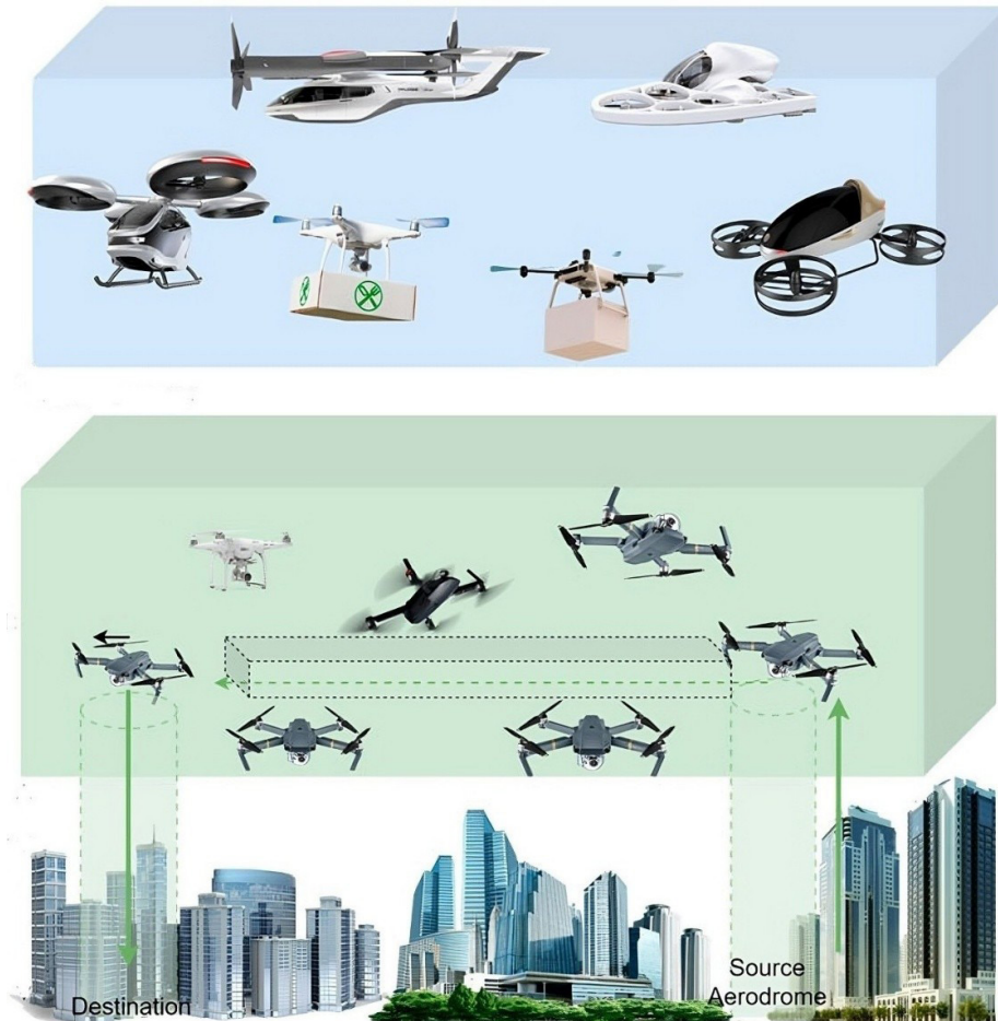
Figure 4: Descriptive diagram (not to scale) of the distribution and use of urban airspace for the UAM. Shrestha et al. (2021)
