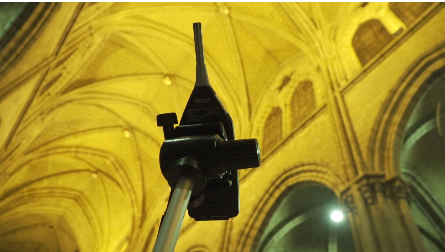
Figure 5: Sound Level Meter and Acoustic Analyser: used to do the RT60 measurement
