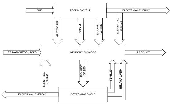
**Figure 2.** Classification of cogeneration systems according to sequence production of electricity and heat.
