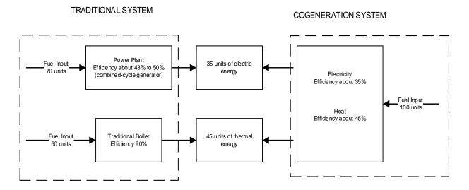
Figure 1. Comparison of energy flow in a traditional system versus a cogeneration system.
