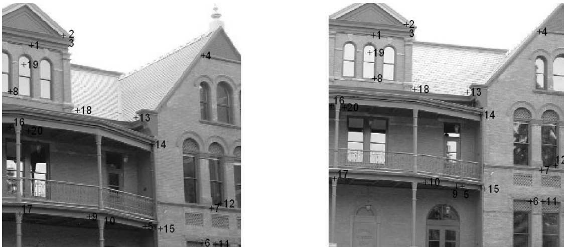
Figure 8. Final matching points using RANSAC to enforce the epipolar constraints in both images.
