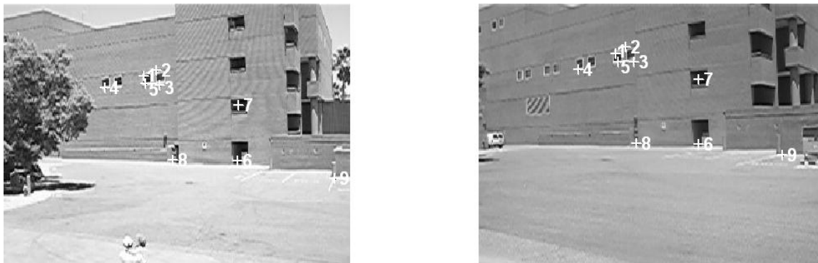
Figure 9. Final matching points applying RANSAC to enforce the epipolar constraints in both images of the example presented in Section 2.
