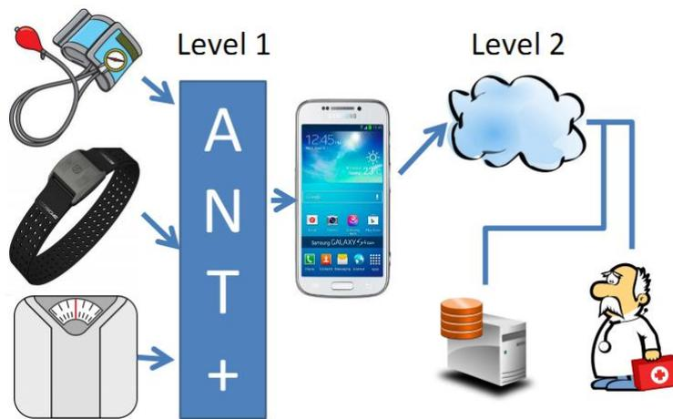
**Figure 2.** Automatic Blood pressure reader, sports heart rate monitor, and radio wireless body composition platform are used in this study. Level 1 communications use ANT+ and level 2 various technologies to reach a remote server on the Internet.
